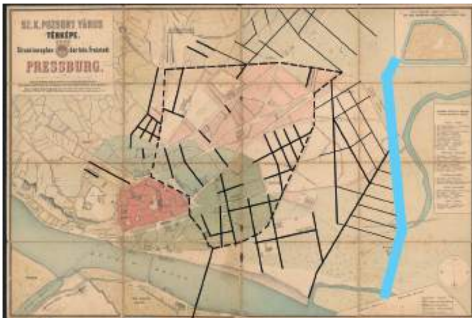
Figure 2: Július Laubner and Technical Department, Regulation Plan, 1906. Newly designed and regulated streets and a water canal outlined in the city plan of 1882. Source: Bratislava City Archives, Collection of Maps and Plans, No. 1045.
