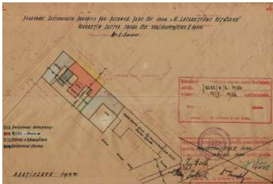
Figure 5: Regulatory plan of Lazaretská adapted to Frič's project allowing courtyard wings to be built and the street wing to be higher, 1935. Source: Bratislava City Archives, Office of the Chief Architect, box 330, ID No. 3210.
